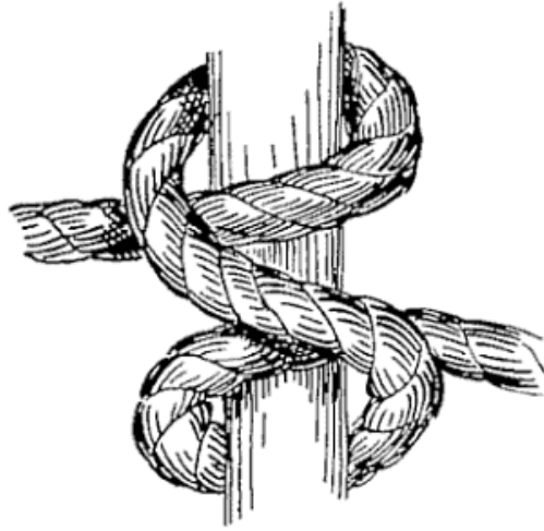
FIG. 36 A.—Clove hitch or builder's hitch (tying).
