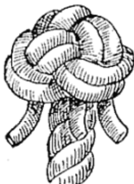
FIG. 126.—Double wall and crown.
