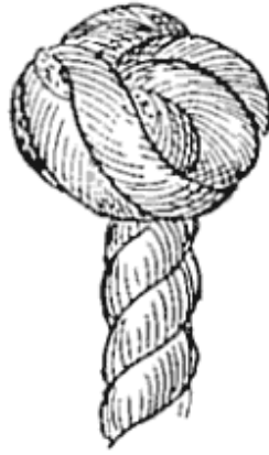
FIG. 123.—Double wall (complete).
