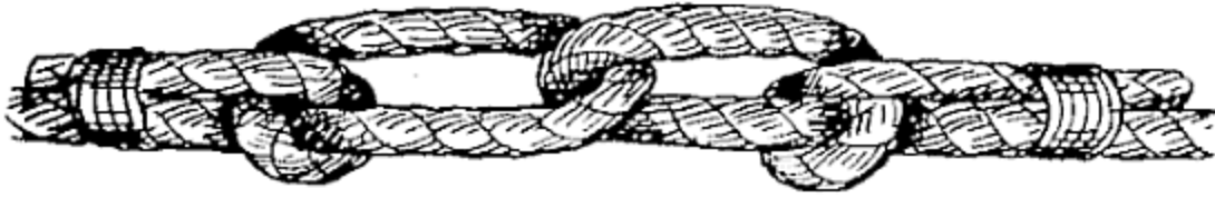
FIG. 29.—Half-hitch and seizing.
