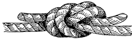
FIG. 19.—Ordinary knot (finished).
