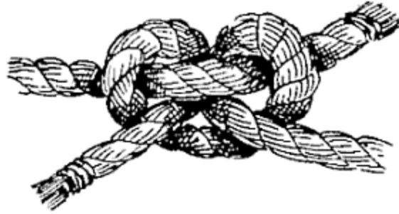
FIG. 14.—Slipped square knot.
