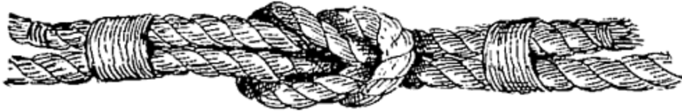
FIG. 15.—Square knot with ends seized.
